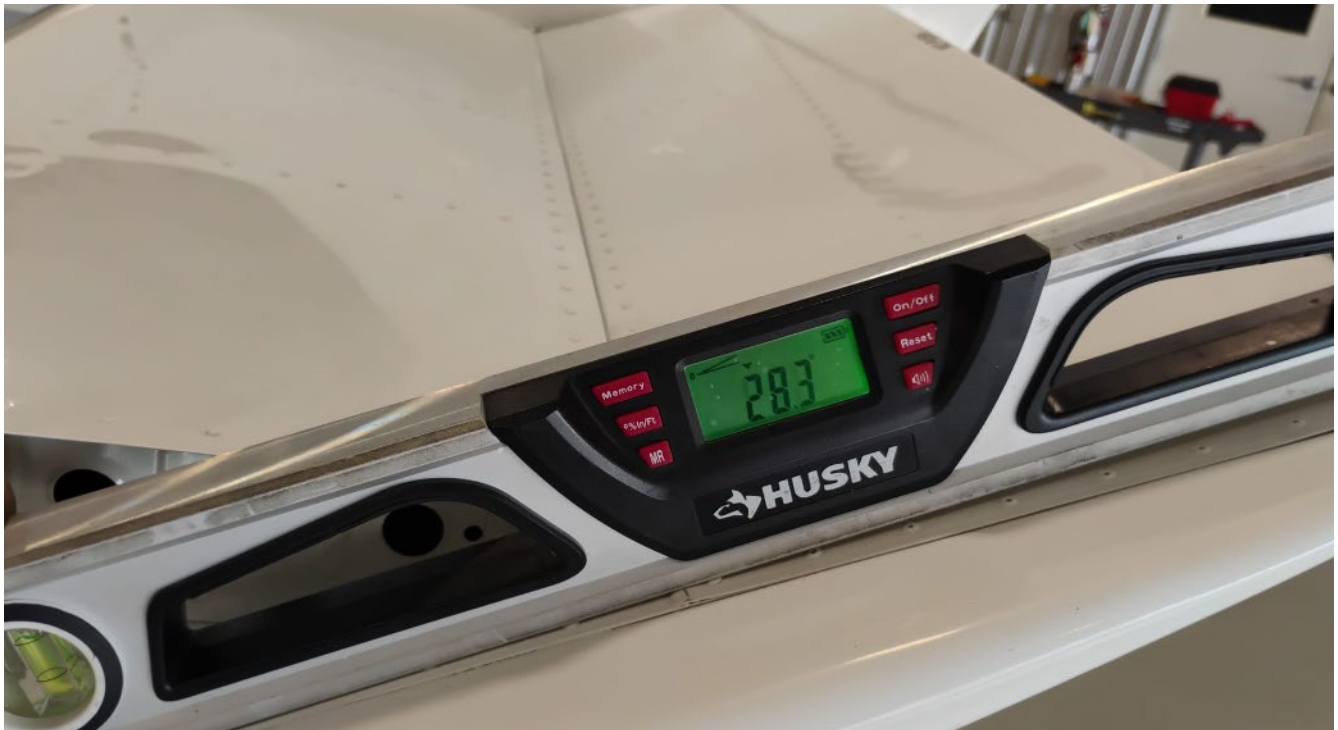
Figure 3.5.2.4. Elevator angle measurement.
