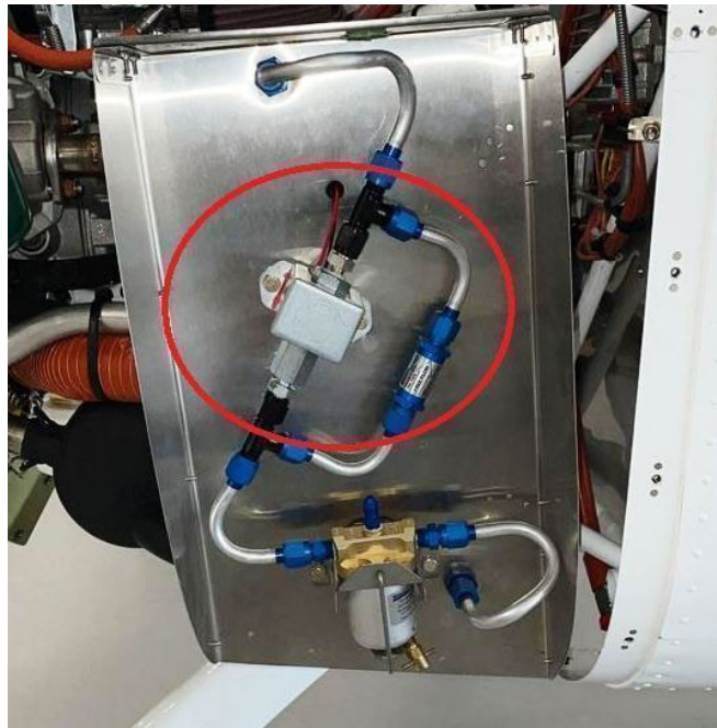
Figure 2.4.6.1. Fuel Pump Installation.
