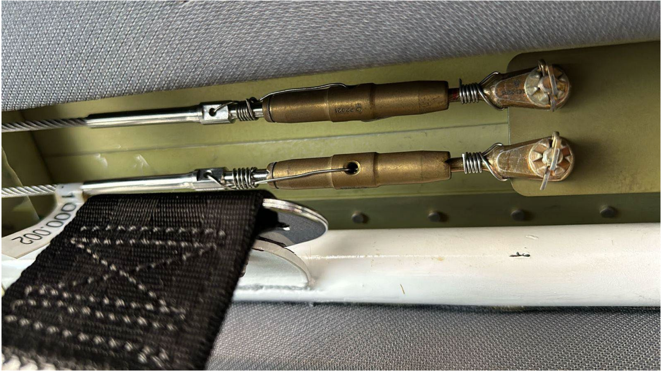
Figure 2.2.2. Tensioning point of the aileron
