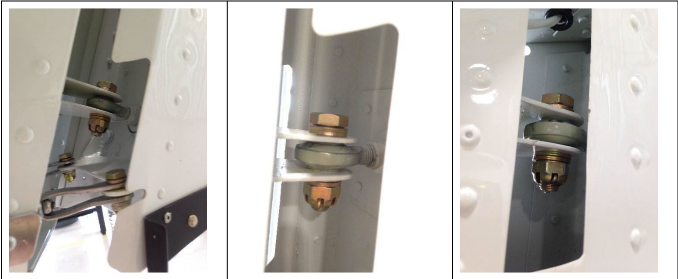
Figure 1.10.2.4.3. Rudder Rod Ends.
