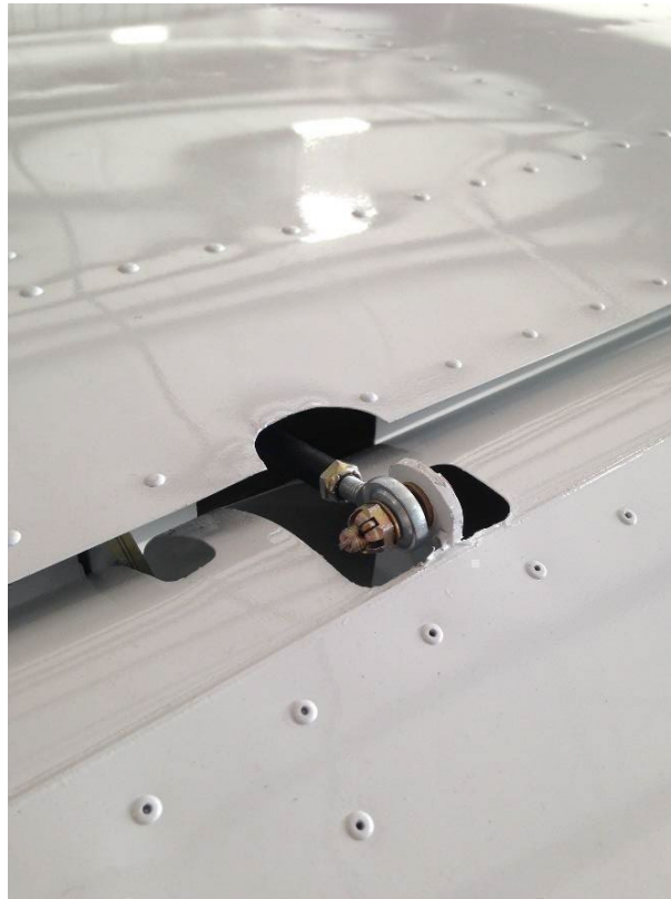
Figure 1.10.2.3.2. Aileron Rod End.
