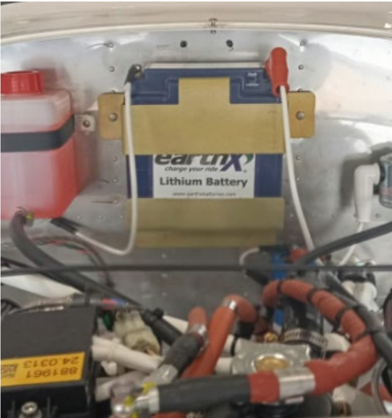
Figure 2.4.8.2. Final Battery Installation.
