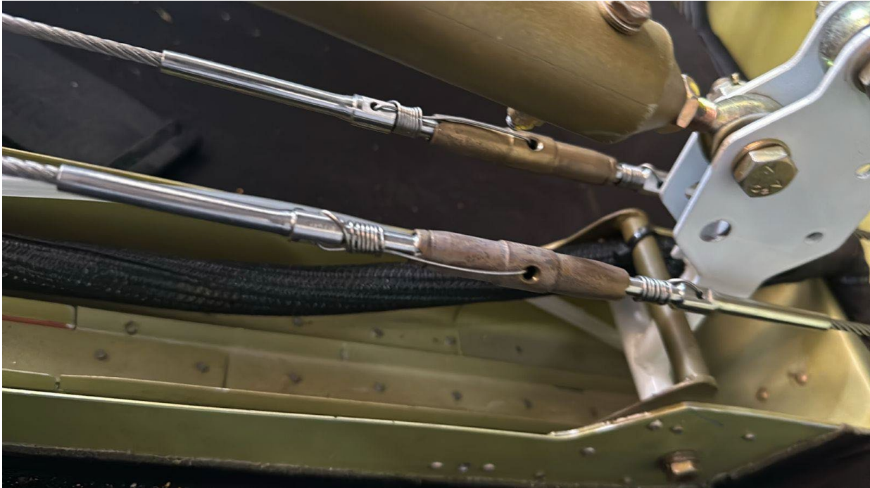
Figure 2.2.2. Tensioning point of the rudder
