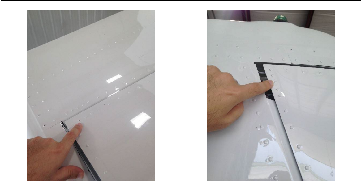
Figure 2.1.7. HT and VT' reference points.
