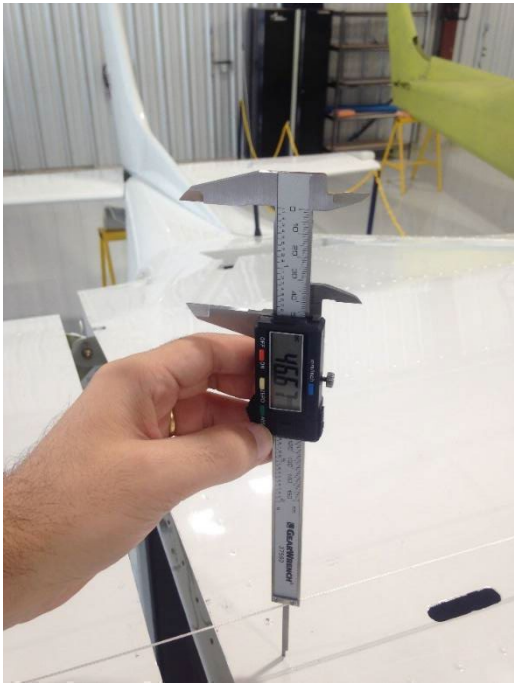
Figure 2.1.4. Height of line at the fuselage.
