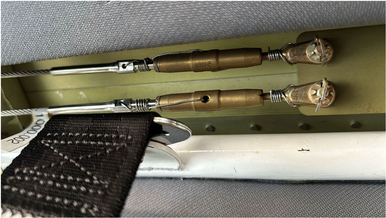
Figure 2.2.2. Tensioning point of the aileron
