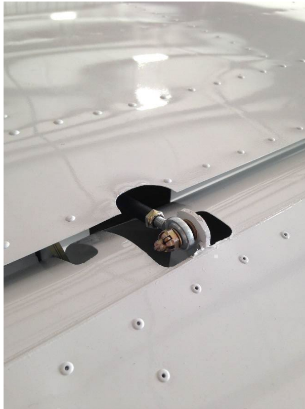
Figure 1.10.2.3.2. Aileron Rod End.
