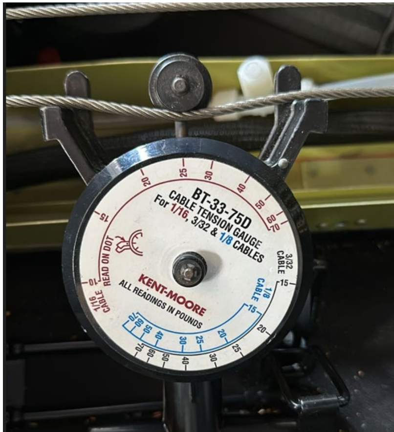
Figure 2.2.1. Measure of the rudder tension cable
