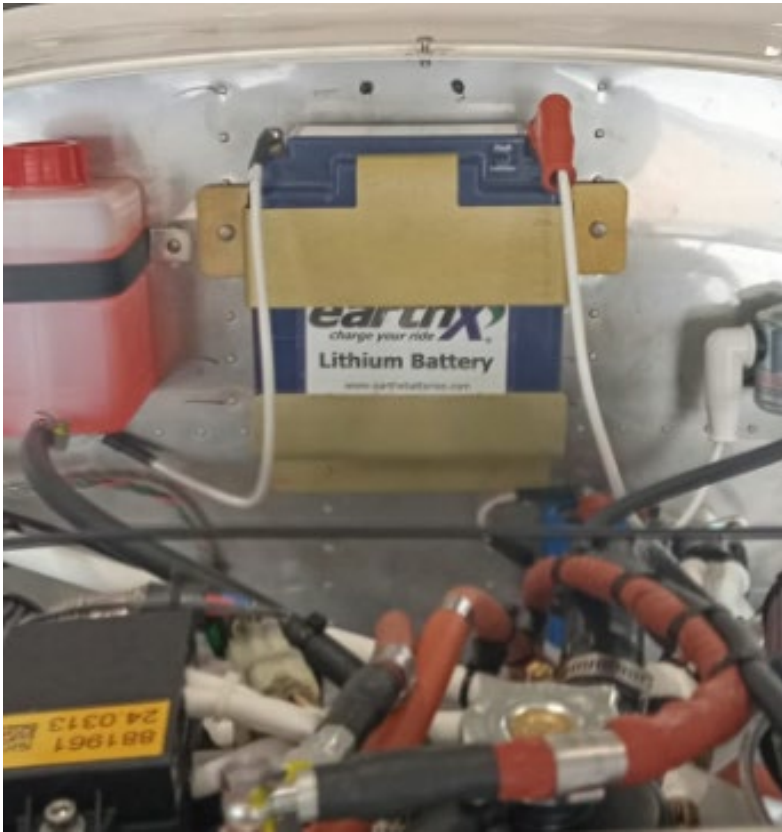
Figure 2.4.8.2. Final Battery Installation.
