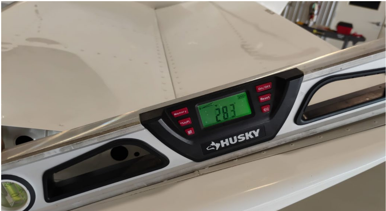
Figure 3.5.2.4. Elevator angle measurement.
