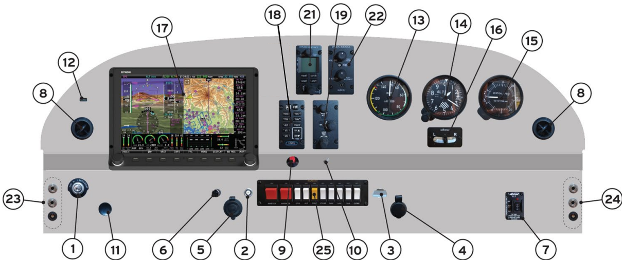
Figure 8.2.1 Instrument Panel for Dynon System
