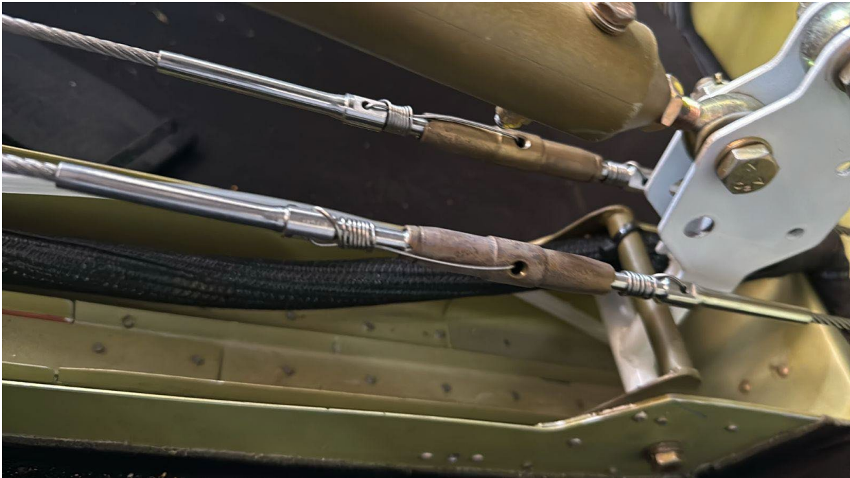
Figure 2.2.2. Tensioning point of the rudder
