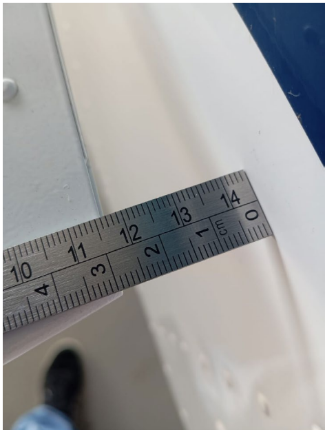
Figure 3.5.3.6. Measured gap at full deflection angle
