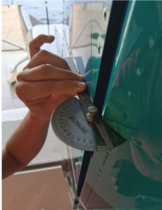
Figure 3.5.3.4. Rivet line measurement
