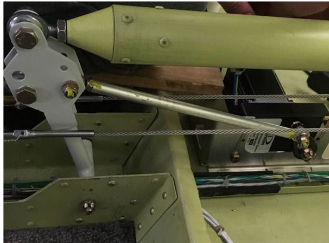
Figure 1.10.2.7.1. Push-rod elevator servo.
