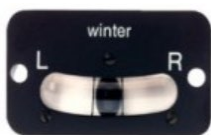
Figure 3.1.1. Slip/skid ball, Digital and Analog installed on the cockpit panel.
