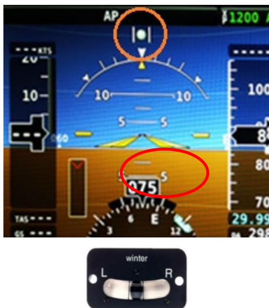
Figure 3.1.1. Slip/skid ball, Digital and Analog installed on the cockpit panel.
