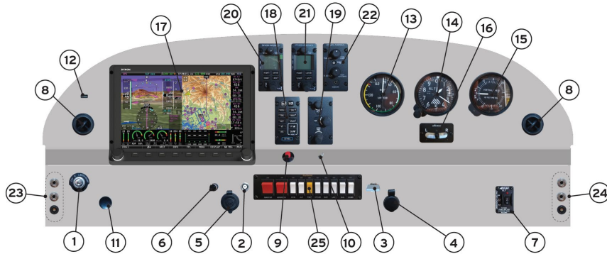
Figure 8.2.1 Instrument Panel for Dynon System
